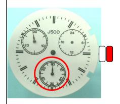
2) FIT THE STOPWATCH MINUTE HAND (EYE AT 10H) AT 29 MINUTE POSITION.
