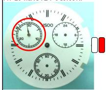
4)FIT THE 24 HOUR HAND (EYE AT 2H) AT 23H POSITION AND TURN THE CROWN CLOCKWISE UNTIL THE 24 HOUR HAND AT 24H POSITION (MINIMIZING BACKLASH). THEN, FIT THE HOUR, MINUTE AND SECOND HAND AT ZERO POSITION.
