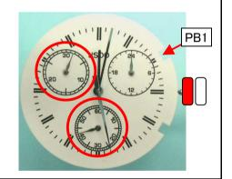
STOPWATCH RESET/CHECK THE ZERO POSITION.
