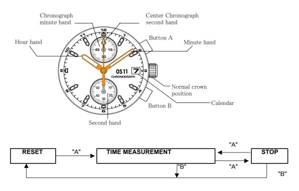
E) CHRONOGRAPH RESET (INCL. AFTER REPLACING BATTERY) This procedure shoud be performed when the chronograph 1/1 second hand do not return to the 0 second position after the chronograph has been reset, and including after the battery has been replaced.
