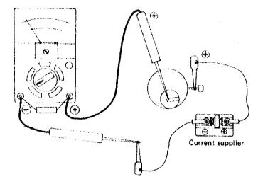
Less than the specified value  $(2.5\mu\text{A})$ : Normal More than the specified value  $(2.5\mu\text{A})$ : Defective
